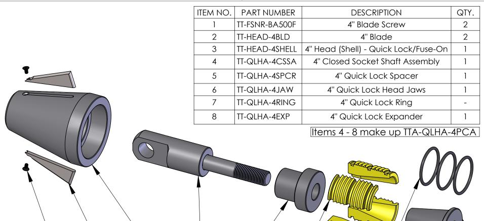
\*\*The 3 Quick-Lock Rings are included with the set of Jaws. Item #7 is the part number for a replacement Ring\*\*
