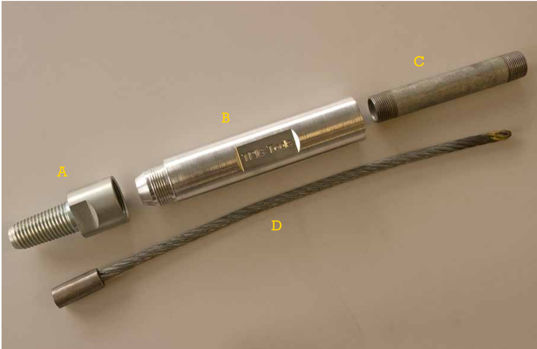
Major components of the TRIC Pusher/Wedge assembly: PE adapter (A), pusher (B), galvanized steel pipe sample (C), and 3/8" aircraft cable or PTI wire (D). For splitting soft material (plastic or copper), the Wedge is used in place of the pusher.
